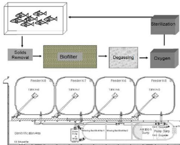
FIGURE 4-2 Recirculating aquaculture system: schematic of a module
