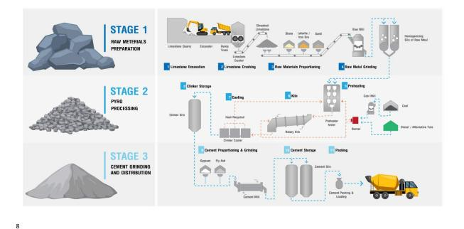
The manufacturing process behind concrete is based on the production of cement since the main component is cement. In order to create concrete a combination of about 10-15% Portland cement and about 15-20% of water is blended and formed into a paste. This paste is combined with aggregates, such as sand, gravel or crushed stone, which constitute 65-75% of the mixture. Upon mixing the water and cement, they bind together, forming a solid mass<sup>9</sup>.
